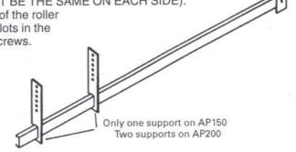
Slide on track support brackets and fasten to a suitable support square to the door and allowing the fall as above with 1 M8 x 40mm coachscrew. (Other supports will be fitted later). Fit rubber Buffers in rearmost track hole and adjust later to correct hole for door open position.
